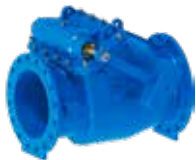
Series 41/36 Swing check valve Metal seated With lever and weight DN350-600 PN10/16 Ductile iron
