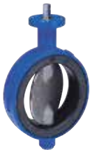
Series 75 Butterfly valve Centric with fixed liner Wafer type DN40-1400 PN10/16 Ductile iron
