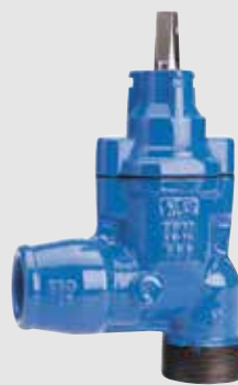
Series 11/30 - angle valve with external thread on inlet and tensile resistant socket joint for PE pipes on outlet.
