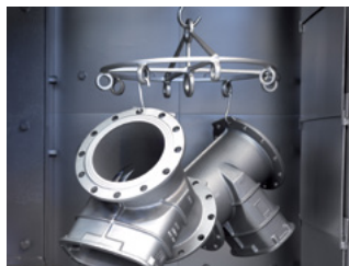
AVK valves are blast-cleaned according to ISO 12944-4
