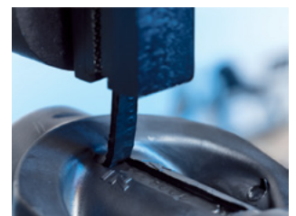
A thin layer of rubber must remain after the peeling test
