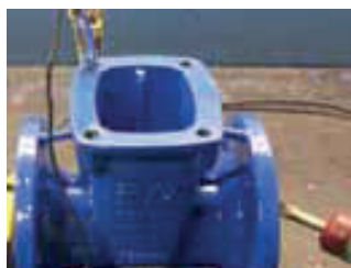
The epoxy layer thickness must be min. 250 \mu on all surfaces
