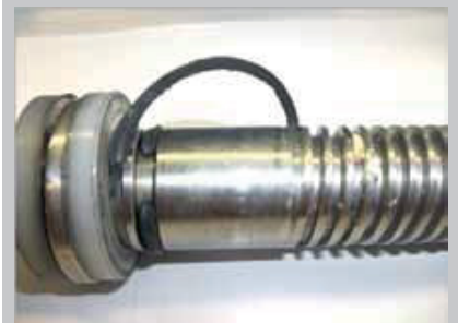
Damaged spindle thread and O-ring
