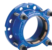
Series 623/10 Supa Plus™ flange adaptor Tensile for PE and uPVC pipes Universal drilling Ductile iron DN40-300 PN10/16
